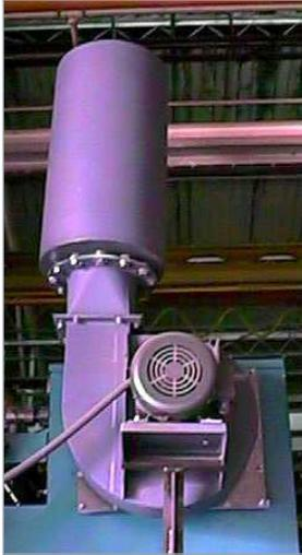
With or without silencers, enclosures offer the maximum level of achievable sound reduction. While this is a significant advantage, it also comes with trade-offs that must be weighed on a case-by-case basis.
